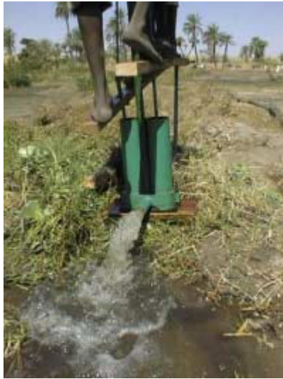
Abb. 5-2 Suction Pressure Pump
